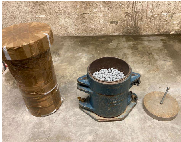
Figure 1. Mold with the grains and weight of 20 kg on the vibratory table to perform the test of e_{min}
